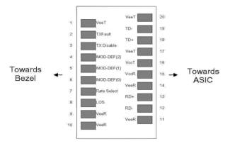
**Pin-out of Connector Block on Host Board**
